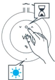
Start the City, press and hold the MODE button until the indicator turns white and stays ON.
