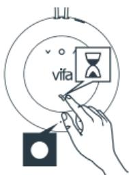
Start the City, press and hold the Mode button until the indicator turns white and stays on.
