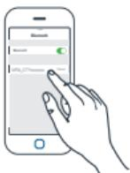
Enable Bluetooth pairing on the device and select VIFA\_CITYxxxxx as the Bluetooth connection device.
